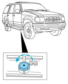
3. Fluid level should be at bottom of the opening.
